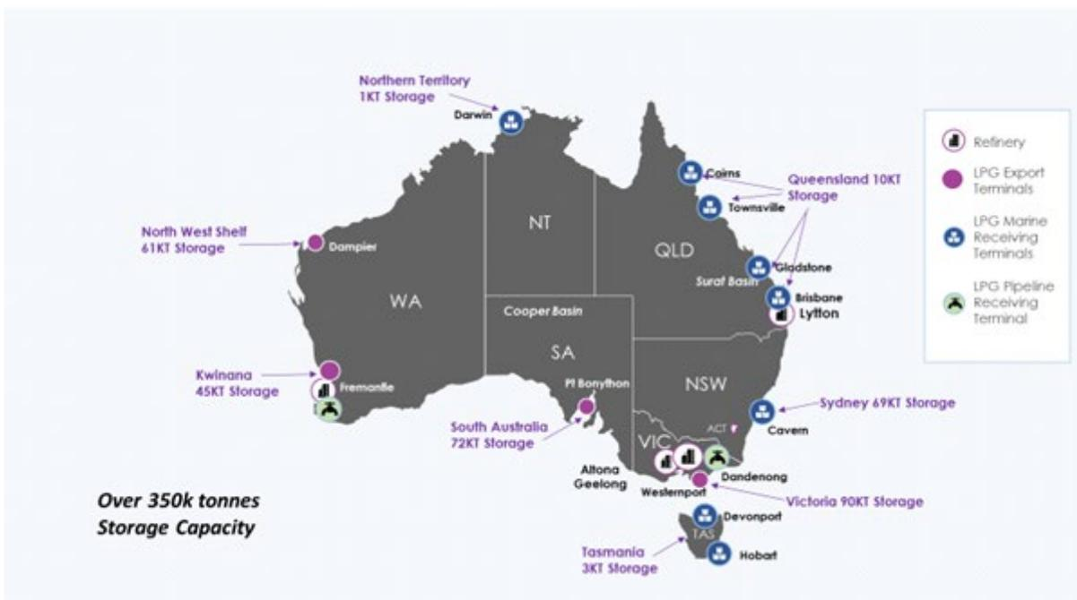
Figure 19 shows that the LPG industry has significant marine port storage capacity – over 350k tonnes.
